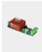
CP.BL Board for buzzer and LED management.
